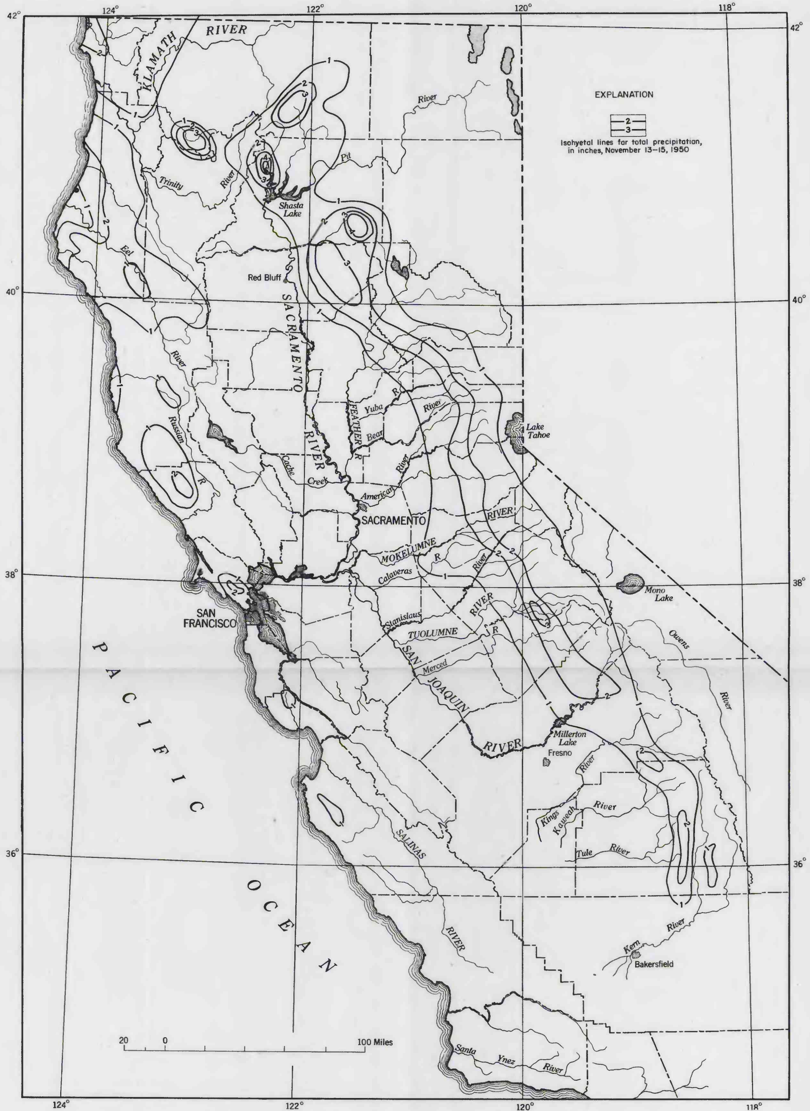
ISOHYETAL MAP FOR STORM OF NOVEMBER 13-15, 1950, CENTRAL VALLEY BASIN, CALIFORNIA
