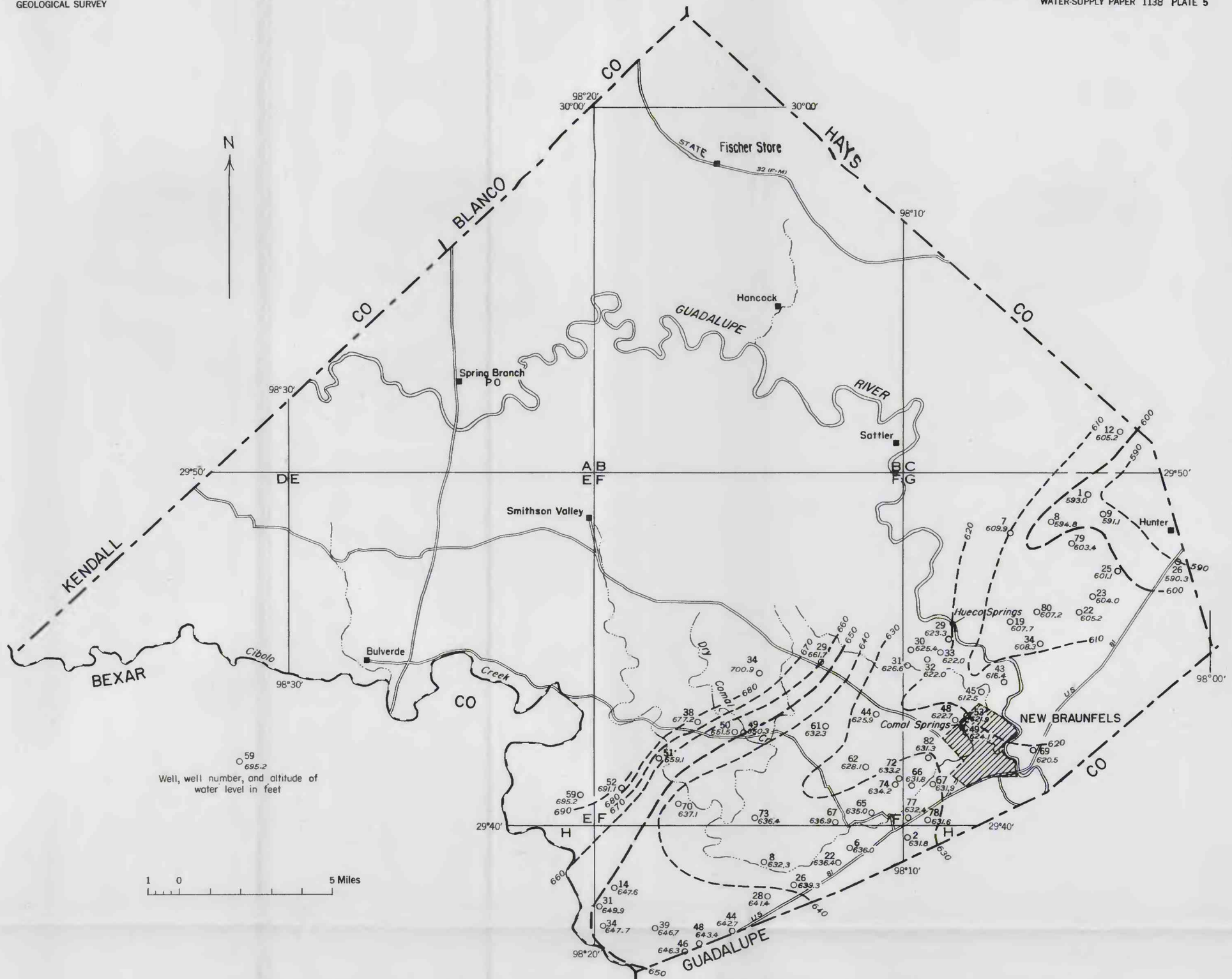
MAP SHOWING ALTITUDE OF WATER LEVELS AND LINES OF EQUAL PRESSURE IN RESERVOIR OF THE EDWARDS LIMESTONE, JANUARY 5-16, 1951
