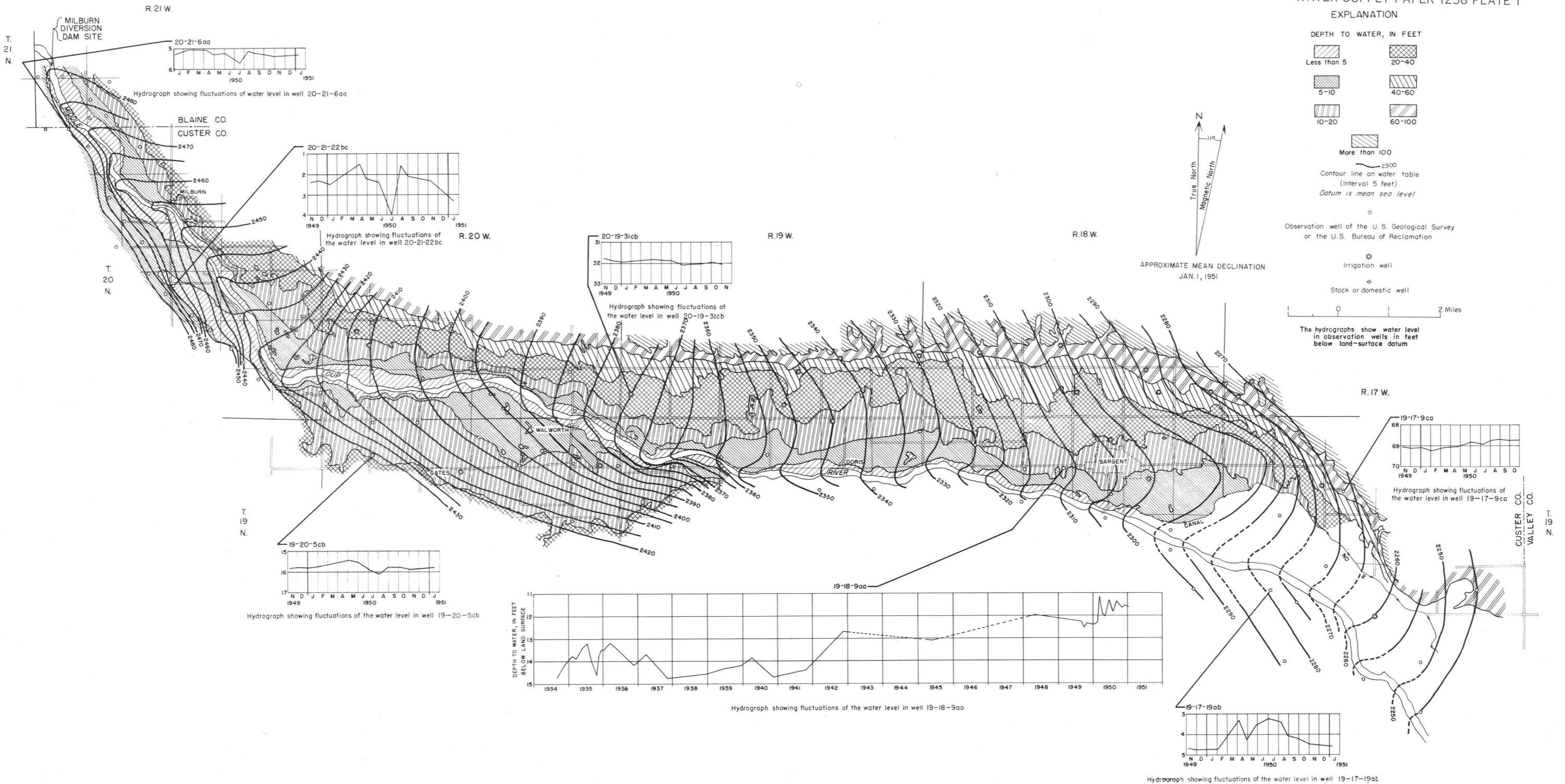
MAP OF THE SARGENT UNIT, NEBRASKA, SHOWING LOCATION OF WELLS, DEPTH TO WATER, AND CONTOURS OF THE WATER TABLE, OCTOBER 1950
