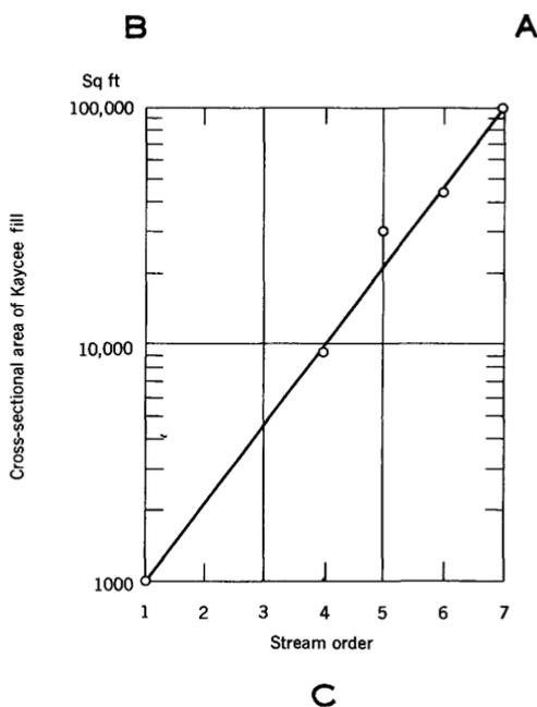
Figure 23. — Cross-sectional area of Kaycee alluvial fill in relation to stream order. Diagram A shows an actual cross section of alluvium above present stream level (black area), and the part of the alluvium eroded away since Kaycee time (hatched area). Diagram B represents the assumed average cross section in the same reach of river. Diagram C shows the relation of computed cross-sectional area by various sizes of stream valleys to stream order which characterizes the sizes of the valley.
