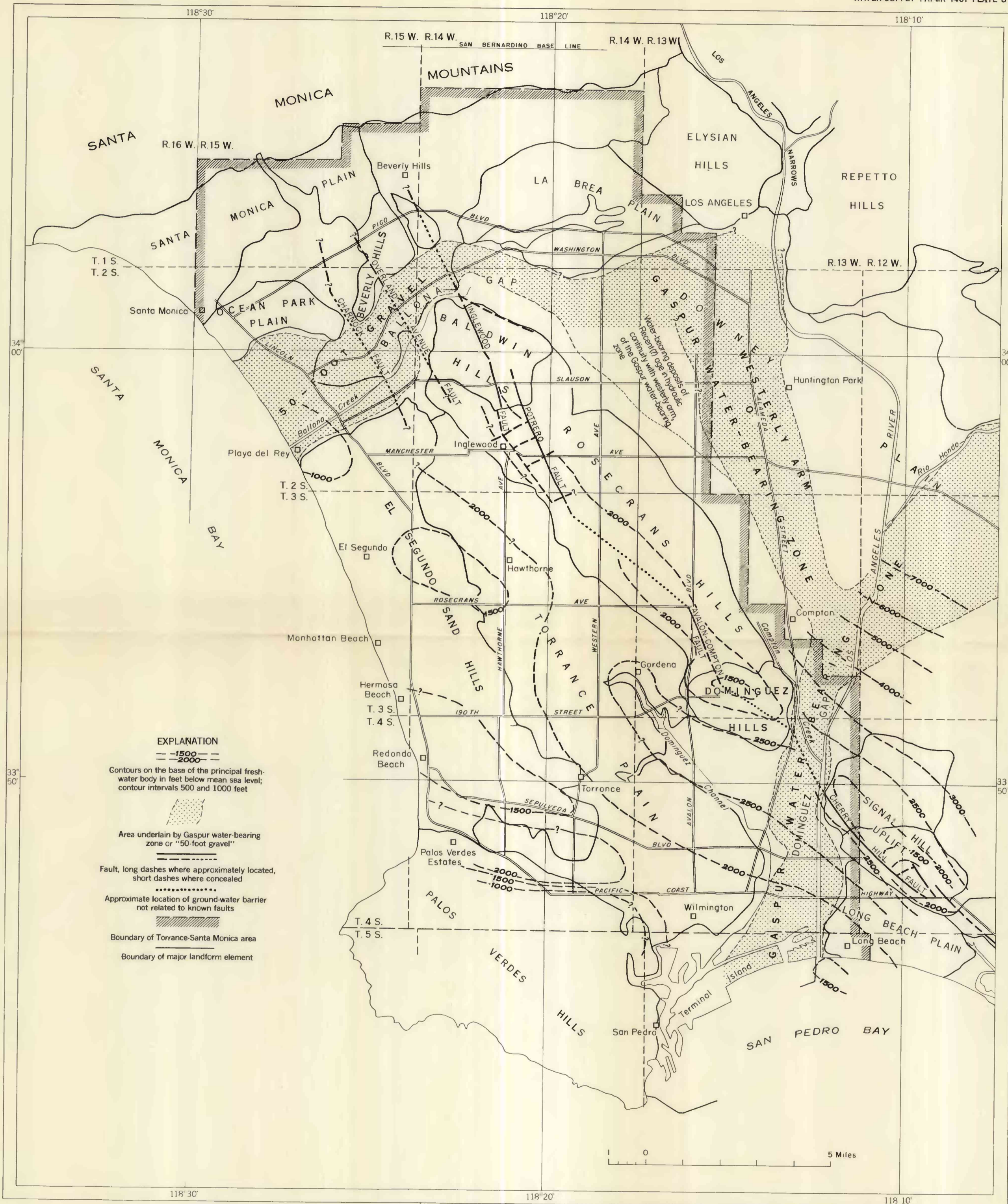
MAP SHOWING GENERALIZED CONTOURS ON THE BASE OF THE PRINCIPAL FRESH-WATER BODY IN THE TORRANCE-SANTA MONICA AREA, CALIFORNIA; ALSO EXTENT OF THE GASPAR WATER-BEARING ZONE AND THE "50-FOOT GRAVEL"
