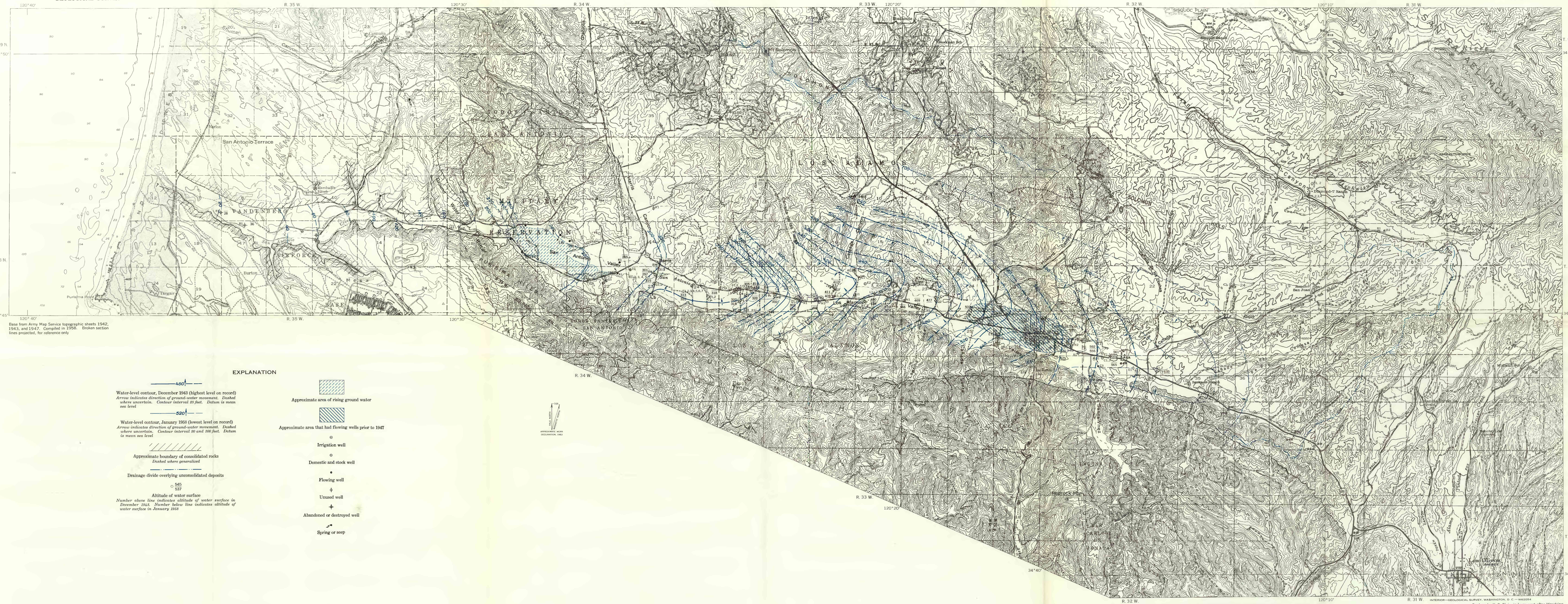
THE SAN ANTONIO CREEK VALLEY AND VICINITY, CALIFORNIA, SHOWING WATER-LEVEL CONTOURS IN 1943 AND 1958 AREA OF RISING GROUND WATER, AND AREA THAT HAD FLOWING WELLS PRIOR TO 1947
