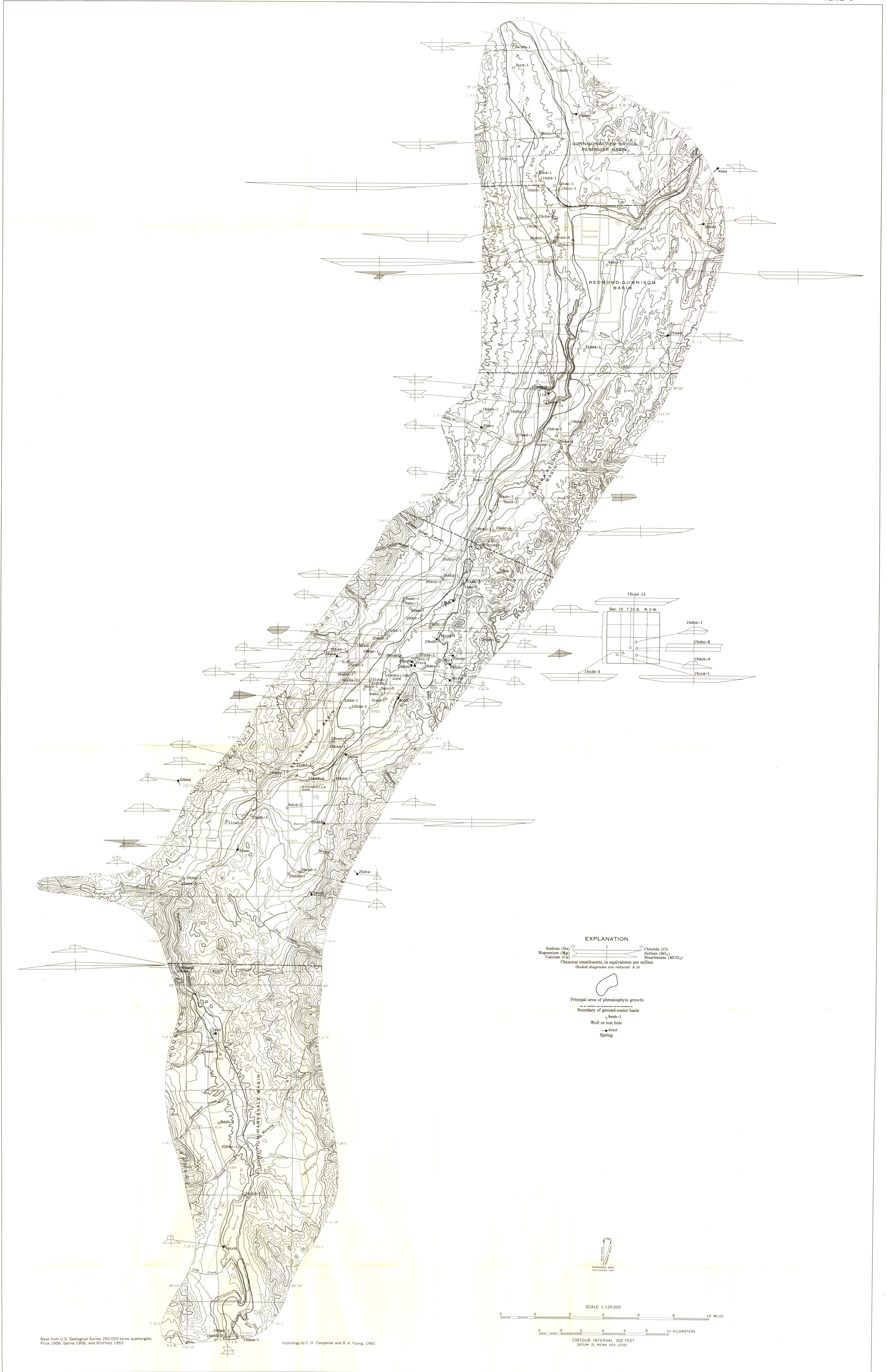
MAP OF THE CENTRAL SEVIER VALLEY, UTAH SHOWING LOCATION OF TRIBUTARIES, SELECTED CANAL DIVERSION DAMS, AREAS OF PHREATOPHYTE GROWTH TEST HOLES, WELLS AND SPRINGS MENTIONED IN THE TEXT, AND DIAGRAMS SHOWING CHEMICAL QUALITY OF THE WATER
