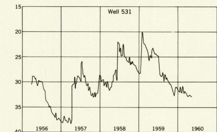
HYDROGRAPHS SHOWING FLUCTUATION OF WATER LEVELS IN WELLS IN THE DAYTON AREA, OHIO
