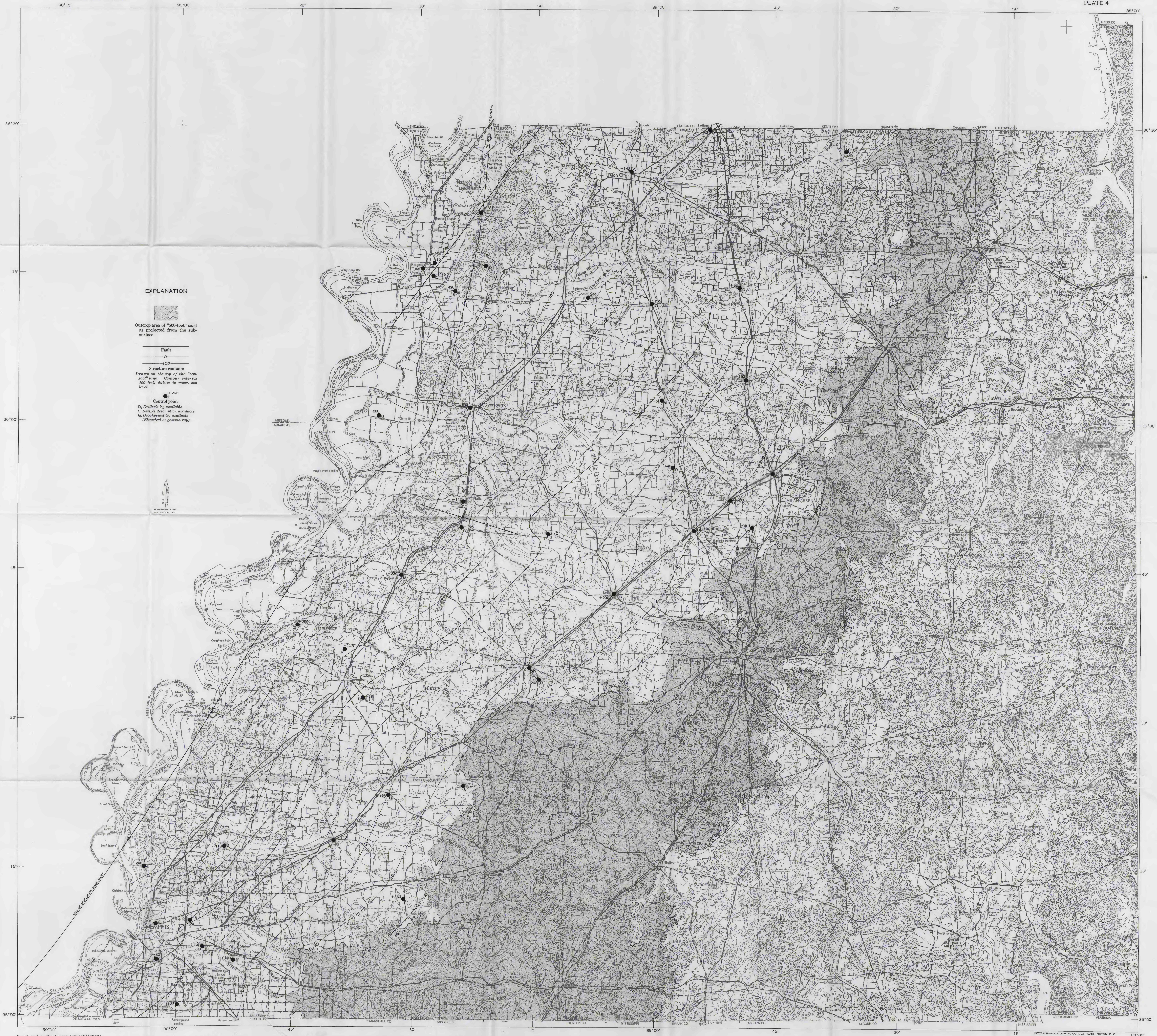
STRUCTURE-CONTOUR MAP SHOWING CONFIGURATION OF THE TOP OF THE "500-FOOT" SAND IN WESTERN TENNESSEE
