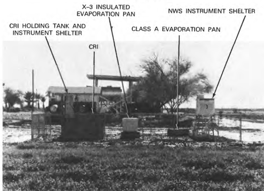
FIGURE 2.—South Station enclosure with Cummings Radiation Integrator and National Weather Service instruments.
