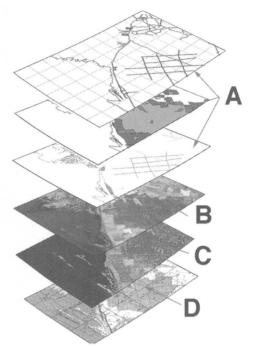
Schematic showing examples of layers that will be contained in the Lake Baikal GIS. A represents Russian thematic maps showing agricultural zones, protected areas, and other land-use data; B shows Russian KFA-1000 satellite imagery with three spectral bands at 5-meter resolution; C shows U.S. landsat TM satellite imagery with seven spectral bands at 30-meter resolution; D is a Russian topographic base map at 1:200,000 scale.
