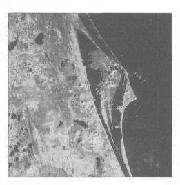
Two images of Cape Canaveral, Fla. Declassified image: KH-5, B&W, 460' ground resolution, April 1963. Current USGS image: Landsat satellite, color IR, 240' ground resolution, March 1992.
